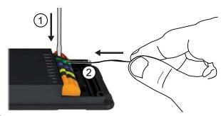
C Connecting LED wires
